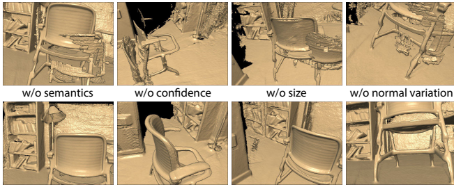
Fig. 3. Effect of different terms of the reconstruction objective. Top row: result without specified term. Bottom row: result obtained with our full method. Note the misalignments present in the top row compared to bottom.
